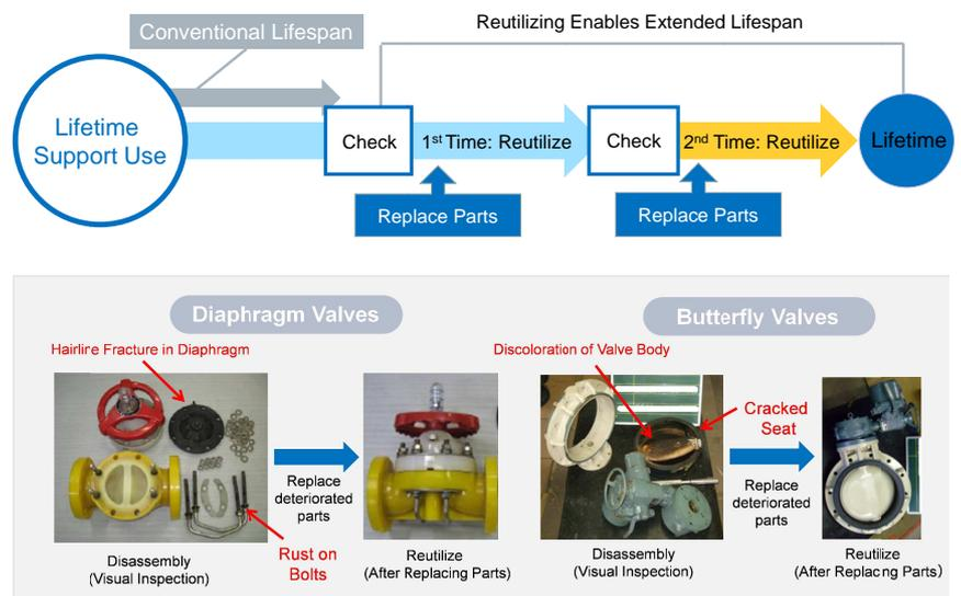
Figure8 .Example of Reutilization via valve lifetime Support
