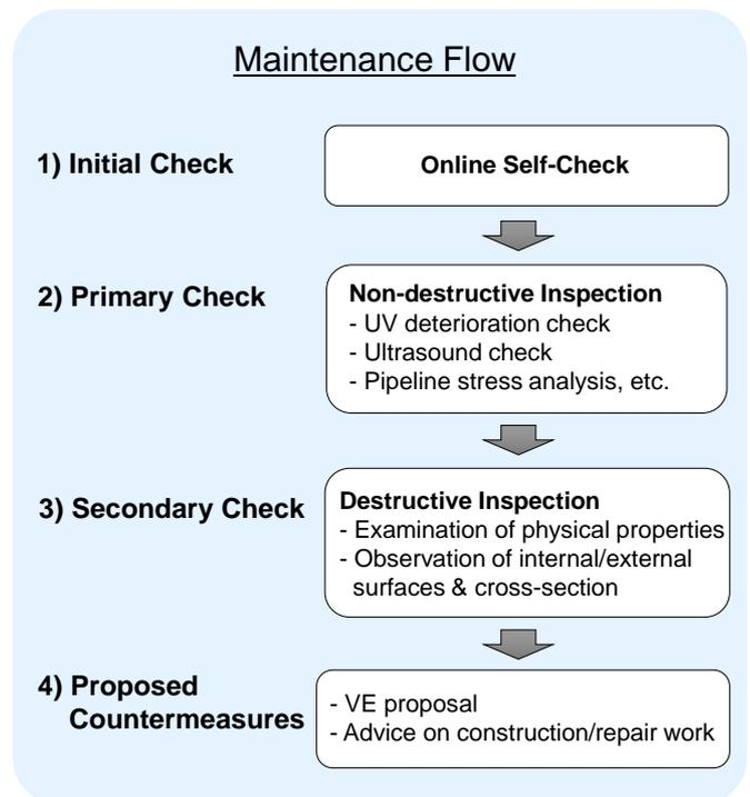
Figure2.Maintenance flow for PVC piping
