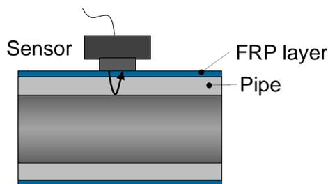
Figure6. Wall thickness inspection using ultrasound
