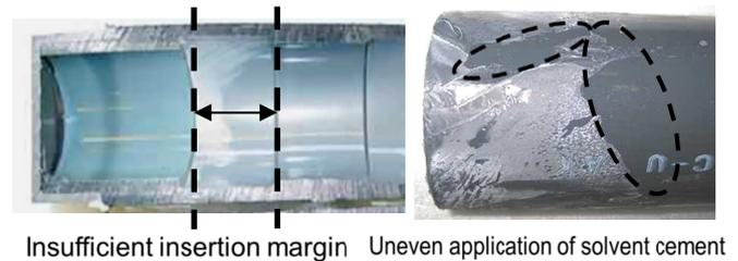
Figure7. Examples of adhesion failure for PVC piping
