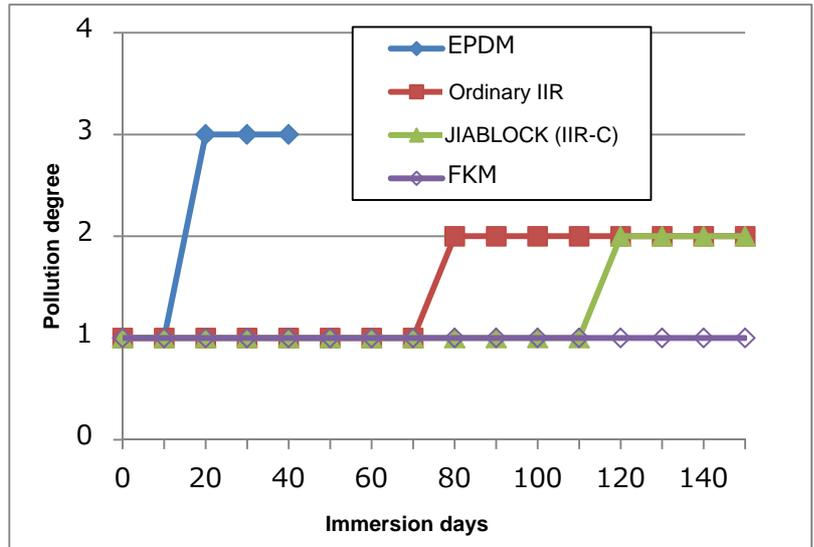
Image 2. Contamination level test
