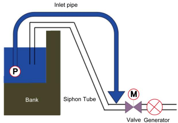
Fig. 1 Outline of Siphon Intake Apparatus
