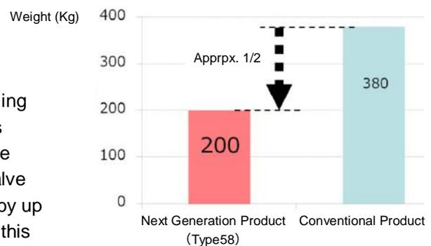
Fig.-3 The difference in weight between the next generation product and the conventional product
