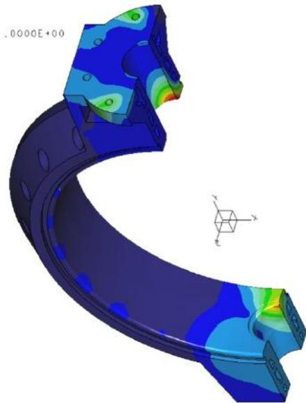
Fig.-2 FEM analysis of the valve body
